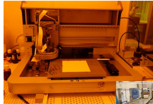
R&R PixDro/MiPlaza S2S 6 inch ink jet engine with integrated dryer
