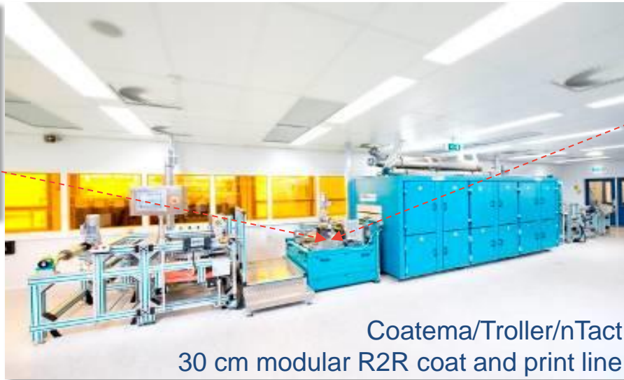
Slot die → together with nTact: R2R intermittent stripe coating
